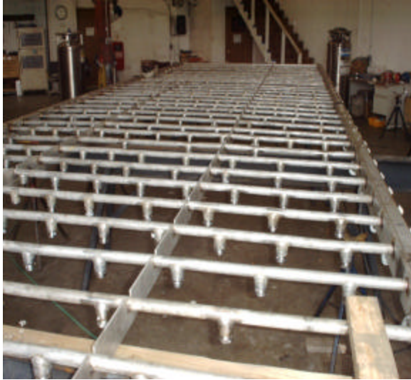
Figure 5: Wet compression nozzle rack before shop acceptance test.
