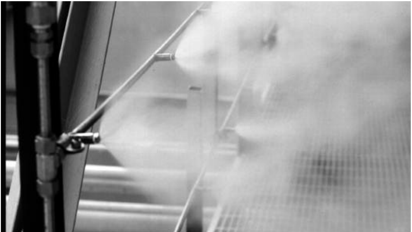
Fig.2: A zone array showing an actual nozzle mounted on stainless steel tubing.
